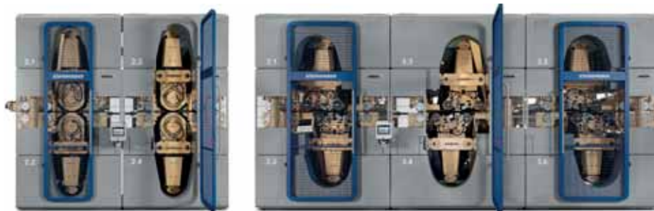
Satos TSQ wide belt sanding machine with five sanding stations
